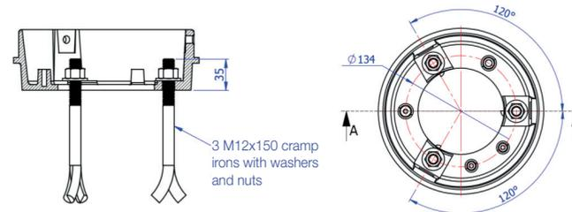
NB: The bollard can be fixed using M12 chemical anchors (not supplied)
