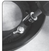
a) disconnect the earth wire (1 H M8x12 screw + washer)
